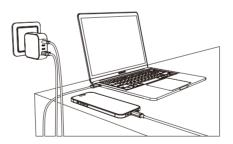
As pictured above, connect the 165W GaN Charger to a Wall Outlet (AC 100-240V).
