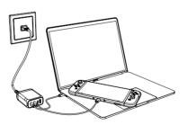
As pictured above, connect the 240W GaN Charger to a Wall Outlet (AC 100-240V).
